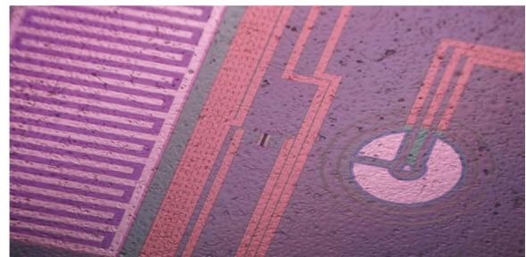
Fig. 2: Area of the chip showing all three types of sensors covered with transformed MSCs
